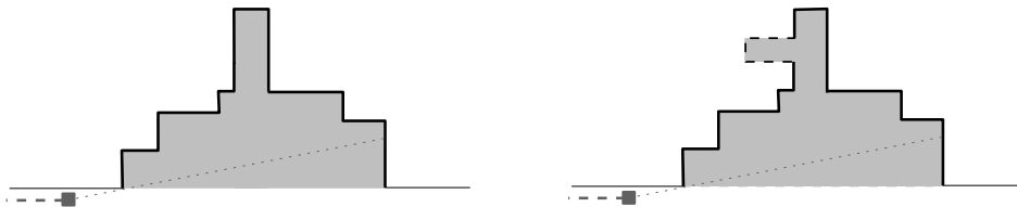
Figure 4: Left: If the dark gray point represent the scan position, a robot with discrete vision cannot see the entire bold sides, resulting in a non-visible region (NVR), shown in gray; an NVR is dealt with by performing a binary search. Right: Within a non-visible region, there may be parts that even a robot with continuous vision may not see completely (dashed), requiring the robot to enter the NVR; one way to deal with such a situation is the introduction of turn adjustments, when the need arises.
