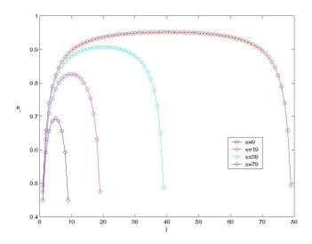
Fig. 2. Multidamping parameter  $\mu_i$  with respect to iteration step i for various values of largest expansion order  $\kappa$  for truncated TotalRank case. It can be seen that the respective Google-type surfer would have to spend most of his time focusing on the existing link structure; however note the abrupt increase (decrease) phases during his first (last) "clicks"; these phases can be the dominant feature for small  $\kappa$ .
