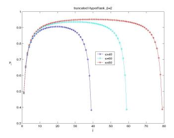
**Fig. 4.** Multidamping parameter  $\mu_i$  with respect to iteration step i for various values of largest expansion order  $\kappa$  for GHR case: Symmetry and behavior are similar to that of TR as expected by the similarity in the corresponding expansions.
