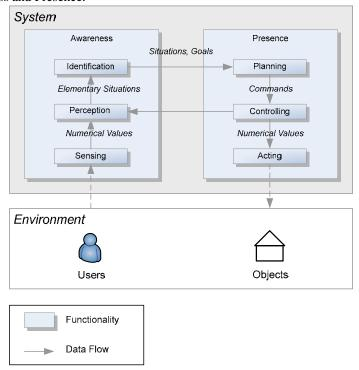
Fig. 2. Functional Blocks of AAL system
