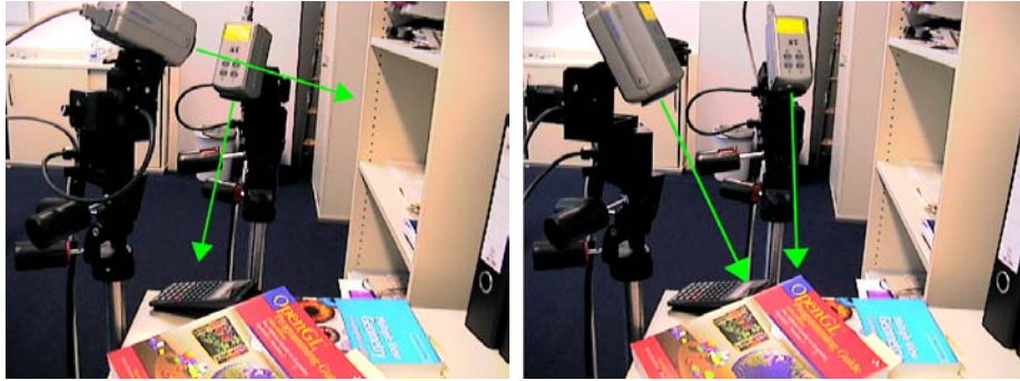
Fig. 1. Example for adjusting the fields of view of two pan-tilt unit cameras to enable an extrinsic calibration.
