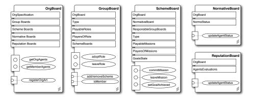
**Fig. 2.** Basic kinds of artifacts in ORA4MAS, with their usage interface, including operations (represented by circles) and observable properties (represented by rectangles with circles in their center), and the link interface (represented by rectangles with circles on their left side)
