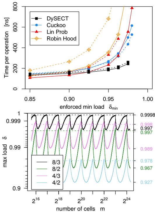
■ **Figure 5** (*left*) Word Count Benchmark. Behaves like a mix of insert and find operations. DySECT’s performance is nearly independent form the load factor. (*right*) Experimental Max Load Bounds. Dependent on the number of cells (different  $B/H$  parametrizations).
