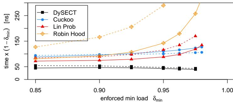
■ **Figure 4** Insertions into a dynamic growing table enforcing a minimum load factor  $\delta_{\min}$ .
