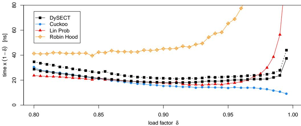
■ **Figure 2** Insertions into a Static Table. Here we show the influence from the load factor, on the performance of insertions. To make insertion time more readable, we normalize it with  $t_{op} \cdot (1 - \delta)$ .
